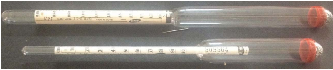
Figure no.1 Alcoholmeters /Acetonometer
